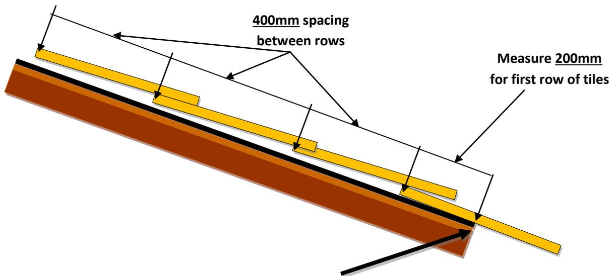
**Roof edge:** Start first row at 200mm. This initial spacing can be **increased** or **decreased** depending on the desired overhang effect.
